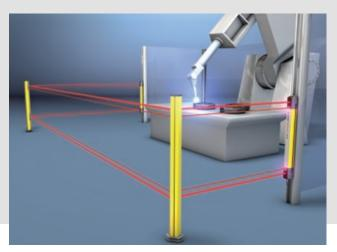
Easy alignment with integrated laser alignment aid when setting up access guarding.
