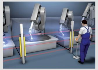
Access guarding with 3-beam transceiver of the MLD 300 series for conveyor and storage systems.
