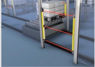
MLD 500 Single Light Beam Safety Devices complement the MLD series and are used, for example, if Multiple Light Beam Safety Devices are not suitable due to the mounting options present at the application site. MLD 500 Multiple Light Beam Safety Device with integrated muting indicator in an AS-i Safety application with sequential muting.
