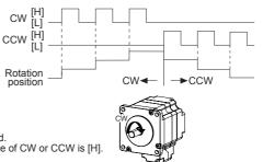
%Do not input CW, CCW signals at the same time in 2-pulse input method. It may not operate properly if another direction signal is inputted when one of CW or CCW is [H].
