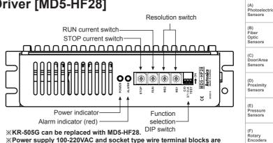
**%KR-505G** can be replaced with MD5-HF28. \*Power supply 100-220VAC and socket type wire terminal blocks are upgraded comparing to KR Series.
