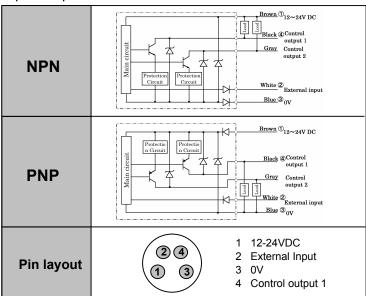
\* Gray line (Control output 2) is only for the 2 output type (D3RF-TD).
